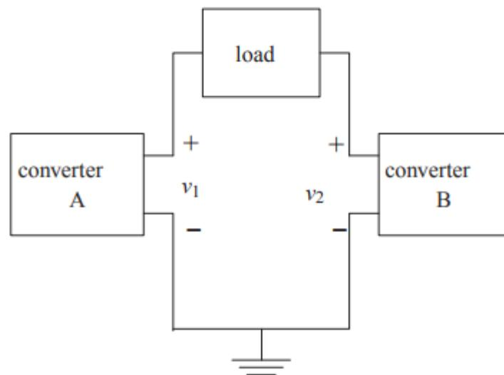
Figure 2: Basic representation of the boost inverter.
