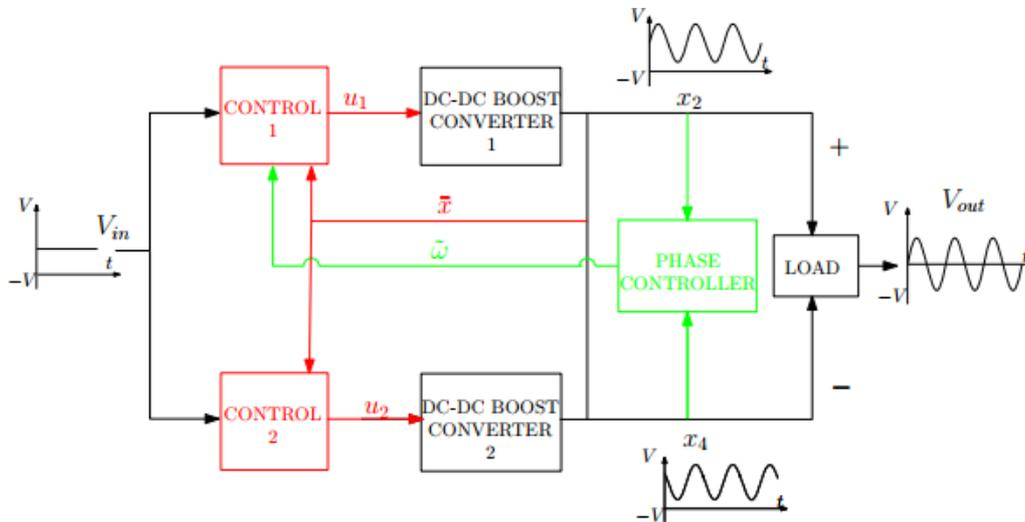
Figure 3: Controlled boost inverter with PHC.
