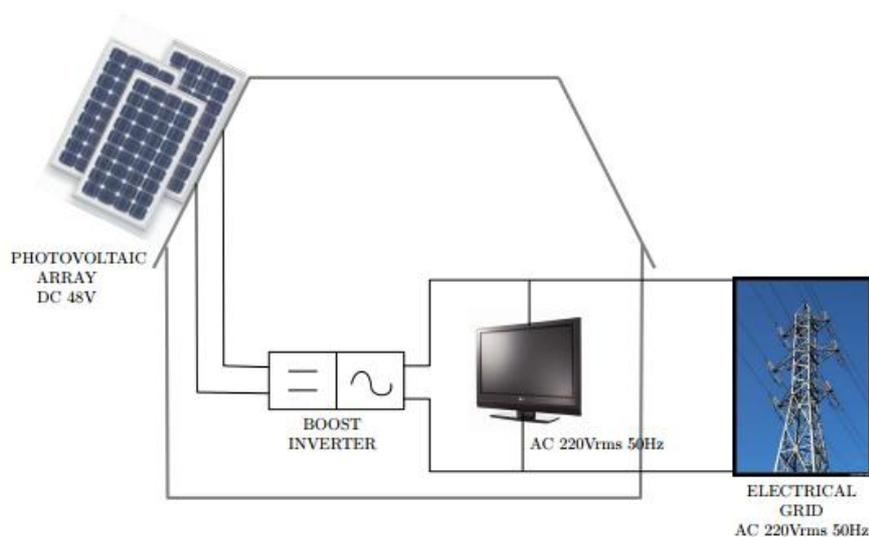
**Figure 1: Domestic photovoltaic installation.**
