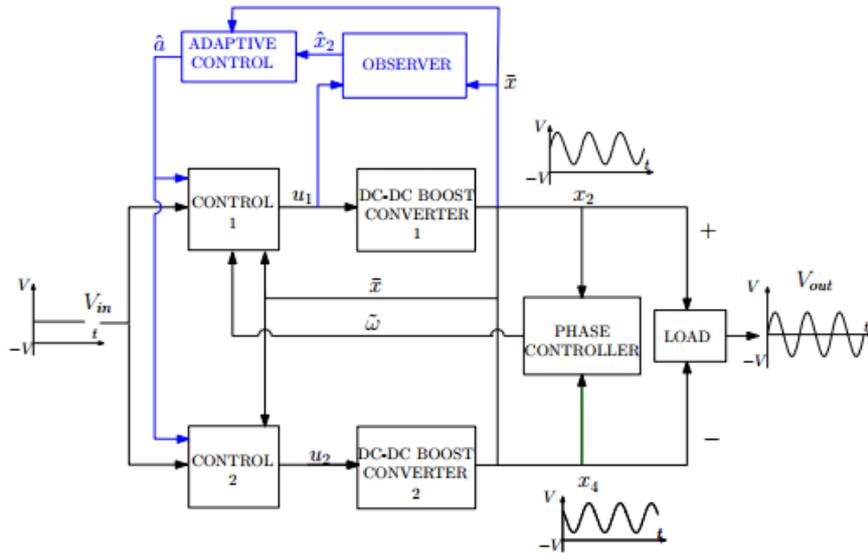
Figure 4.1: Controlled boost inverter with observer
